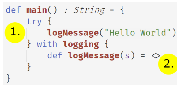
(c) Triggering the operation wraps the source of the logging effect in a handler (1.). A hole is used to allow type checking without implemented effect operations (2.).
